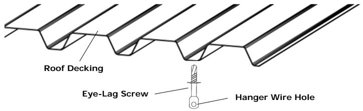
4. Attach ceiling hanger wire to eye-lags. Each full length main runner should be supported in at least 3 places by hanger wire. Make certain that a hanger wire is attached to each corner where lights will be located.
