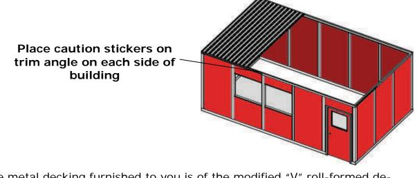
The metal decking furnished to you is of the modified "V" roll-formed design. As such, it will grow or shrink in width during assembly. Care should be exercised to control the dimensions while erecting. Make sure that all walls are plumb as you begin fastening the roof deck to the ceiling cap.
