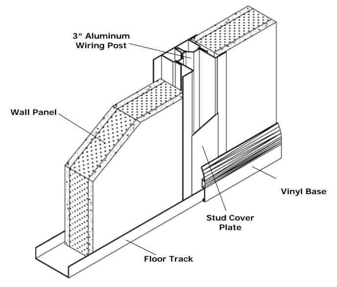
Note: For load-bearing or 2-story applications, Inplant Offices will provide a 14ga plate measuring 8" long by 3" wide to place inside the floor track under every wiring post.
