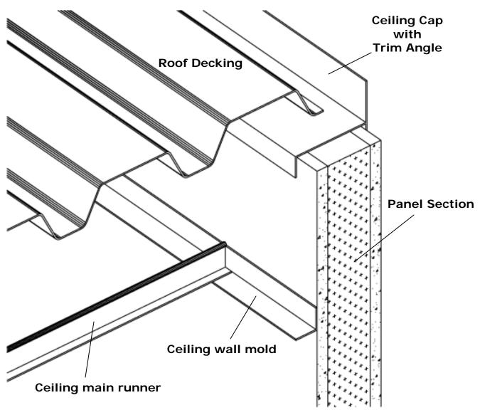
The standard ceiling furnished is the 2'x4' lay-in suspended grid type. The installation is similar to other applications of this type of system.
