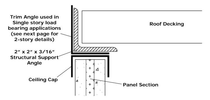
SECTION VIEW OF STRUCURAL SUPPORT ANGLE FOR 3" SYSTEM
