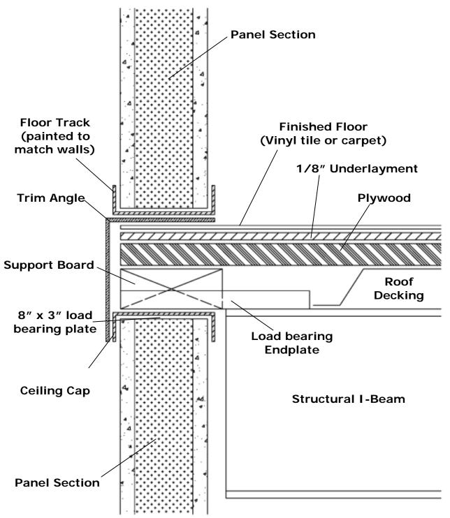
These heavier beams are supported by plates welded to the top of the beams. These plates rest on the ceiling cap and are attached with self-tapping screws. The roof deck must be attached to the support beams on 6" centers.
