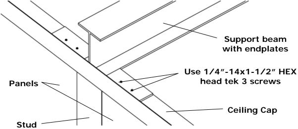
These support beams will rest on top of the ceiling cap. Drill 3/16" diameter holes, two on each side of the beam and attach to the ceiling cap with 1/4"-14x1-1/2" hex washer head self-tapping screws which are provided.
