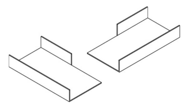
8. Anchor floor track using fasteners (not furnished) appropriate for field conditions and floor compositions. One fastener should be placed in each corner through the lap joint. Other fasteners should be spaced nominally 3' on center around perimeter, plus two on each side of door openings and at both sides of joints.
