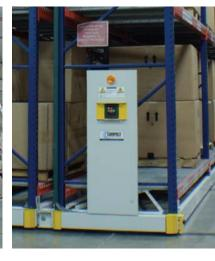
Above: When users pushes a button on the ActivRAC control panel to open the desired aisle, they gain access to any one of the three levels of pallet racking that make up each 65-foot-long carriage. Items can be accessed from either side of an open aisle.
