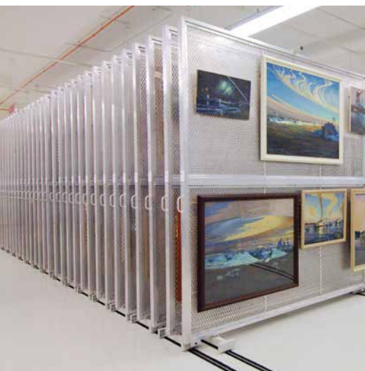
(Above) Tall pallet racks on a Mechanical-assist mobile system maximize vertical as well as horizontal space in the Equipment Vault. (Left) Mobile Art Racks nest together on double rails for optimal compression in the Paintings Vault.
