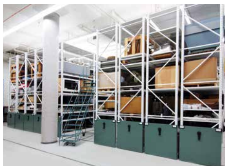
(Above) Tall pallet racks on a Mechanical-assist mobile system maximize vertical as well as horizontal space in the Equipment Vault. (Left) Mobile Art Racks nest together on double rails for optimal compression in the Paintings Vault.
