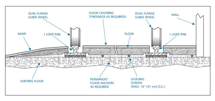
SPACESAVER L FLOOR AND RAMP COMBINES A LOW PROFILE RAISED DECK BETWEEN THE SYSTEM'S RAILS, THAT FEATURES LEVELING SCREW ADJUSTABILITY AND PERMANENT FLOOR ANCHORS, AND A MINIMUM SLOPE ENTRY RAMP FOR A FLOOR AND RAMP SYSTEM THAT IS USED WITH L LOAD RAILS AND PROVIDES UNIFORM FLAT SURFACES THAT WILL ACCEPT MOST FLOOR FINISHING MATERIALS.
