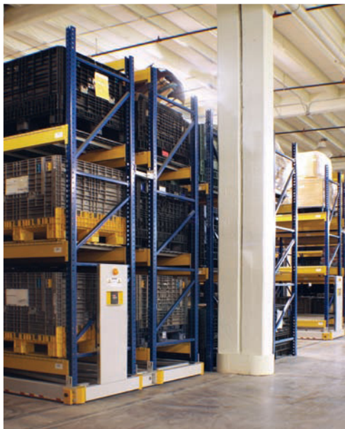
Mobilized storage systems with existing pallet racks
