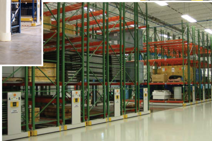
These systems mobilize existing pallet racking and industrial shelving by mounting them onto industrial grade-carriages with capacities of up to 60,000 lbs. per back-to-back rack section. These carriages then travel on rails or tracks that are embedded into the floor.
