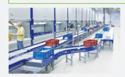
For quick picking and consolidation of orders, the connection of work zones via conveyor systems is an ideal solution. Items are delivered automatically to the access opening, picked and then placed into shipping containers on the conveyor.
