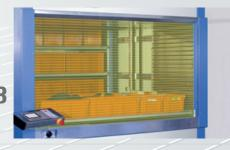
When the shutter doors open to deliver or retrieve a tray the safety light curtain located at the frong of the access opening is activated. If the safety light barrier in front of the access opening is interruped, all movement of the device is stopped immediately for operator safety.
