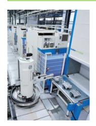
The full tray extraction feature was designed for the handling of heavy and bulky goods that often require the aid of a lifting device. Using full tray extraction, the tray is automatically pushed out onto an extraction table mounted to the front of the VLM for loading and unloading. Trays can also be loaded onto the optional transport cart for safe and easy handling.
