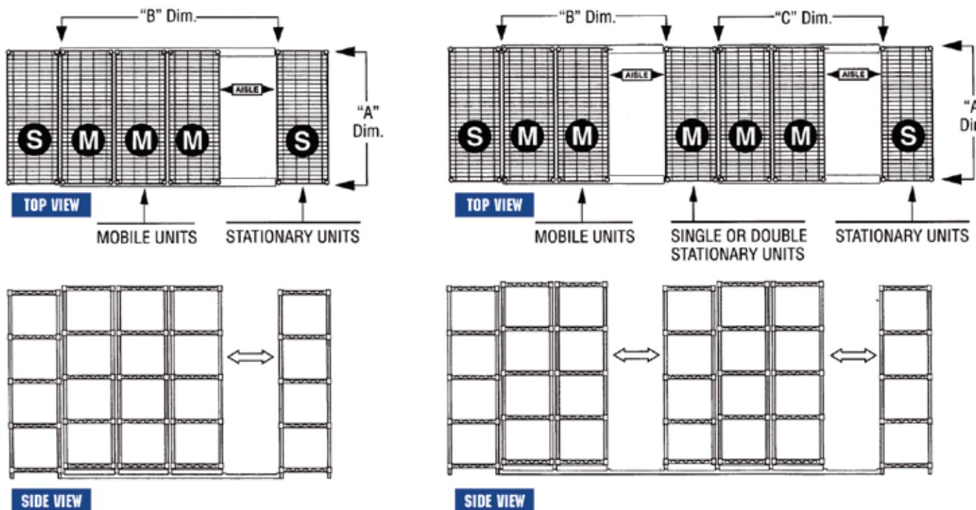
Stationary units at the end or center of a high density system are not a requirement for our track shelving system.
