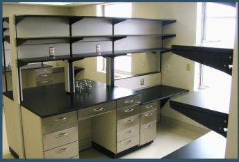
Multifunctional Laboratory Benches These powder coated steel cabinets with stainless steel drawer fronts and chemical epoxy resin tops incorporate gas, vacuum, water, data and electrical lines into each bench for total changeability.
