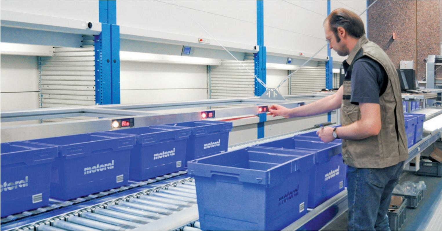
The amount of order picking locations and pick-to-light displays and the buffer capacity are determined by customer specific demands.
