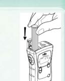
Press eject button and to open door insert the sampler cartridge into the luminometer. Close door and press black button on front of unit to obtain results.
