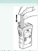
Press eject button to open door and insert the sampler cartridge into the luminometer. Close door and press black button on front of unit to obtain results.
