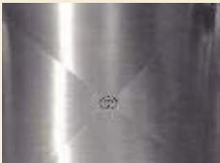
Floor is cross-broke and angled to middle with small holes to drain.
