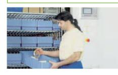
Paperless picking is possible without changing the business processes. The warehouse management system combines several orders into a picking batch via PC control to reduce the number of drive cycles.
