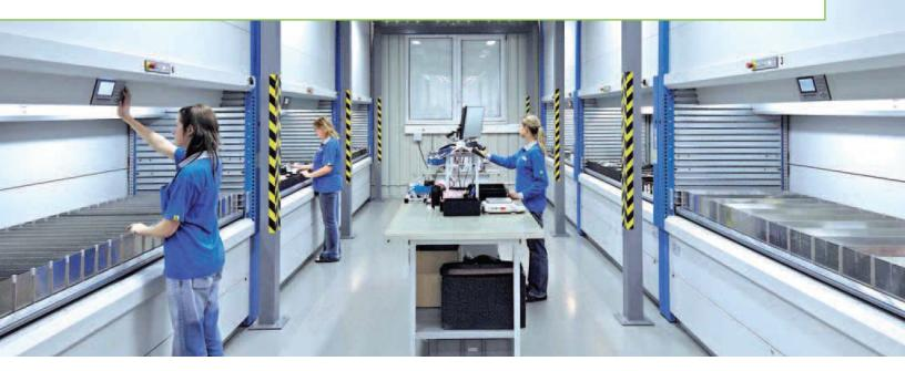
The Kardex Remstar Shuttle XP is an automated high bay warehousing system with a modular design operating on the "goods to person" principle.
