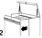
When filing or retrieving, roll the drawer out of the main cabinet to a point where about two inches of the pins remain in the posts of the cabinet.
