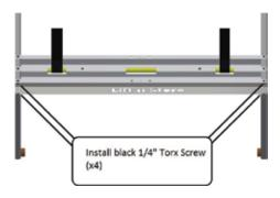
With the super bracket installed on the hanging arms, you can install the nameplate. The nameplate attaches to the top of the hanging arms and super bracket and is held on by 4 black  $\frac{1}{4}$ " Torx screws.
