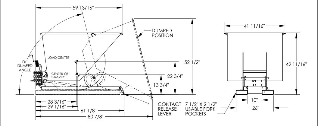
STANDARD FEATURES MODEL NUMBER: SMS-46A-HD-100-LD VOLUME: 1 CU. YDS. CAPACITY: 2,000 LBS. OVERALL WIDTH: 41 11/16" OVERALL LENGTH: 61 1/8" OVERALL LENGTH: 61 1/8" OVERALL HEIGHT: 42 11/16" PULL CABLE IS AT LEAST: 48" TOUGH BAKED IN POWDER COATED BLUE FINISH
