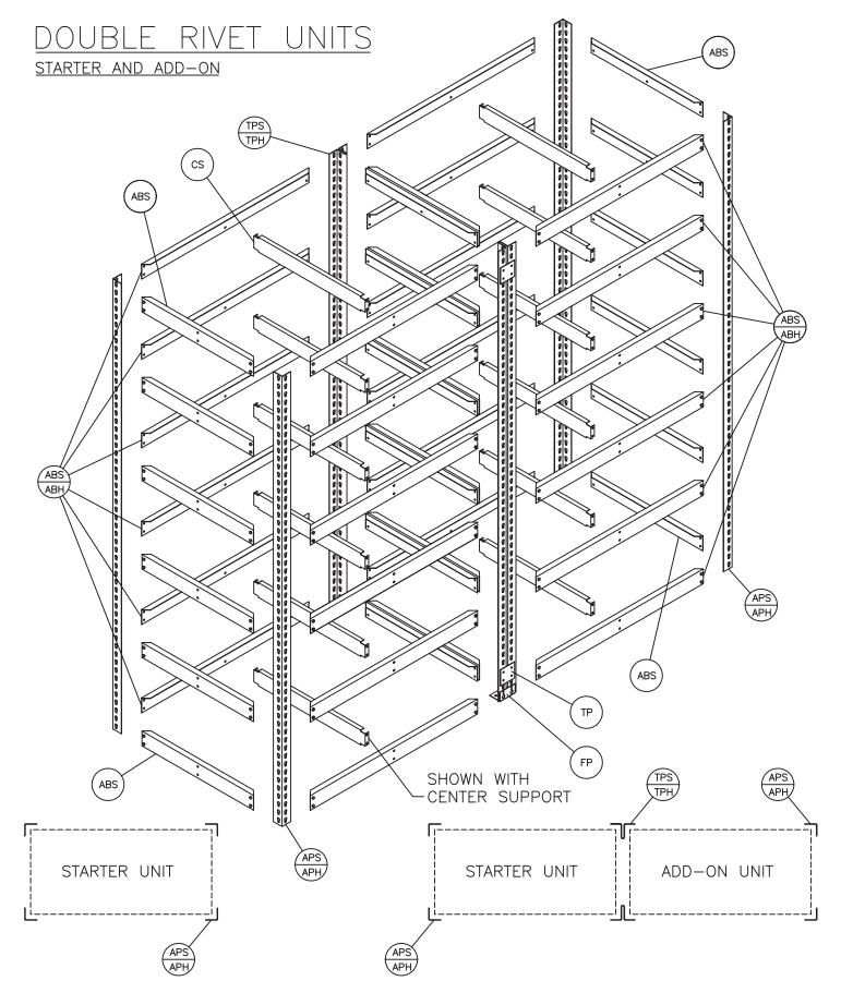
NOTE: WHEN ORDERING HEAVY-DUTY-ANGLE BEAMS UNITS, FRONT TO BACK BEAMS ARE STANDARD ABS BEAMS.
