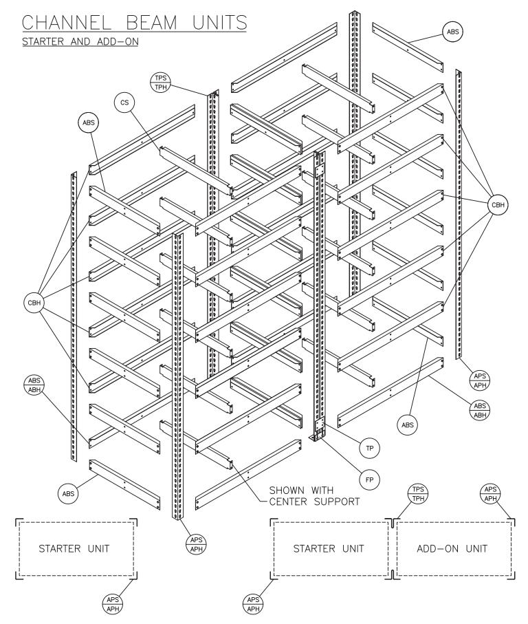
NOTE: WHEN ORDERING CHANNEL BEAM UNITS, ALL BOTTOM LEVEL BEAMS AND ALL FRONT-TO-BACK BEAMS ARE STANDARD ABS ANGLE BEAMS.
