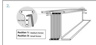
Line up brakcet on end panel to the holes on the outside piece of panel bundle. Screw two bolts into each bracket on the end of the panels as shown.
