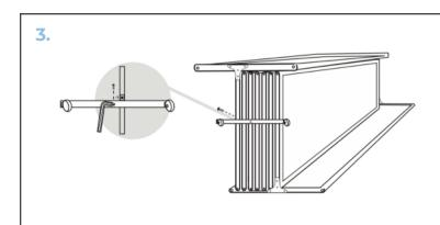
Screw wheel base to bottom of panels into square nuts. Image shows approximate placement. The bottom of panels are predrilled. Slide square nut to this location. Attach wheel assembly with large screw using allen wrench. Keep pressure on wheel bar will help to maintain perpendicular placement.
