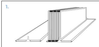
Gently place both end panels on the ground and lift partition bundle (placing it on it's side) on top of one of the end panels.\*
