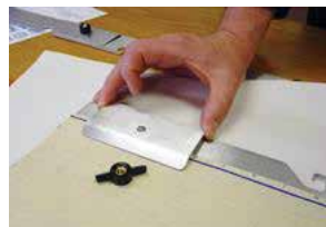
2. Place aluminum posi-grip clamp on post.
