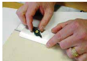
3. Install and tighten knob on post. * Caution: Do not over-tighten knobs.
