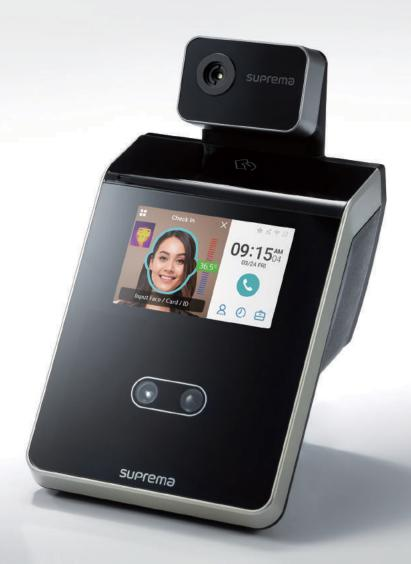
Facial Recognition Terminal 2 with Temperature Detection combines face recognition terminal\* with Thermal Camera to detect users with elevated skin temperature.
