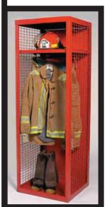
tion of locker contents. The base model is constructed of a 16-gauge steel frame, back, top and bottom, with our tough 2" x 1", 10-gauge wire mesh welded onto the side wall frames. A heavy load capacity, 16gauge steel shelf is mounted 12" from the top of the locker with two coat hooks and a coat rod secured below.
