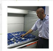
Employees are able to pick the right part in a fraction of the time as with manual picking with the help of light-directed picking, as well as automated batch picking and kitting.
