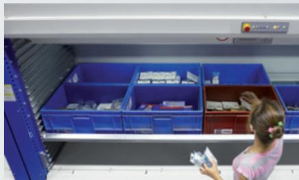
Side walls of the access opening are equipped with shelf rails, enabling the VLM to position more than one tray in the access opening. Also, individual users can adjust the delivery height of the tray to match their physical height providing true ergonomic working conditions.
