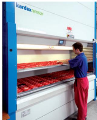
A dual tray delivery option makes it possible to use two work levels in the access opening. A tray is delivered into the first work level in the access opening and the shutter door closes. While items are stored or removed, the next tray is being retrieved and kept in a waiting position behind the access opening, decreasing wait time even further.
