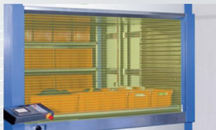
When the shutter doors open to deliver or retrieve a tray the safety light curtain located at the front of the access opening is activated. If the safety light barrier in front of the access opening is interrupted, all movement of the device is stopped immediately for operator safety.
