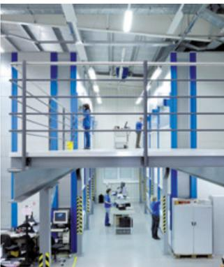
Vertical Lift Modules can be built through several floors with up to 6 access openings placed on the front or rear side of the unit. A mezzanine floor can be installed to enable operation on several levels at the same time (with loading at one level or side and retrieval at the other).
