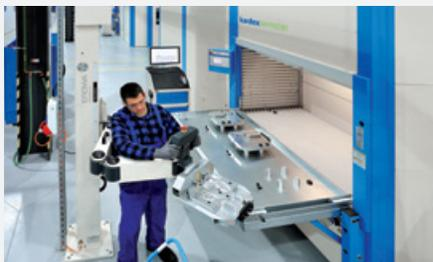
Easy integration of hoists, cranes, grippers and manipulators provide additional ergonomic material handling.
