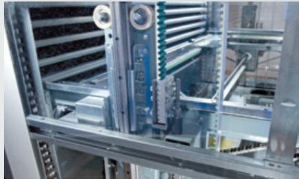
The extractor delivers the requested tray to the access opening or returns a tray to a location within the unit at fast speeds. Both vertical and horizontal travel speeds can be adjusted to accommodate sensitive items.
